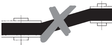
Axial misalignment of sheaves
